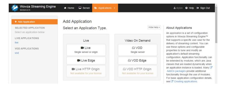
In the default installation of Wowza, we often have the "live" application enabled. All we need to do is choose a stream name "SE5820". Some RTMP servers require authentication. If so, enable "RTMP Authentication" and provide the account and password.
