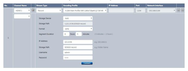
Once the verification is done, click the "Play" icon to start streaming and recording. It is safer to access the recording files on NAS server after you have stopped streaming. To retrieve the files from NAS, open "Computer" or a file explorer window. Enter the server address with two leading backslashes \\\\\10.1.9.56\) and press Enter.
