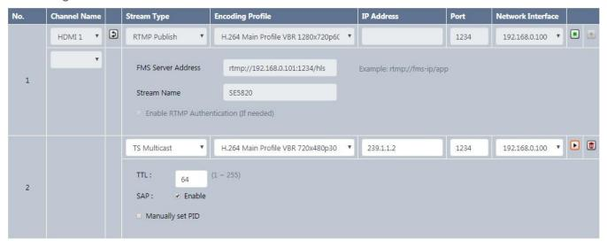
Under "Broadcast List" tab, the two streams share the same video and audio input (HDMI 1). The first stream is sent to RTMP server for transcoding and dispatching while the second stream is sent to local network to players.
