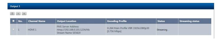
RTMP server can do a lot more than just dispatching the media content. So the playback URL may not be the same as the one displayed under "Output Location". To be sure, consult your service providers or operators for detail.
