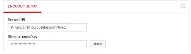
Copy the "Server URL" to "FMS Server Address" and the "Stream name/key" to "Stream Name" in SE5820. Leave "Enable RTMP Authentication" unchecked.
