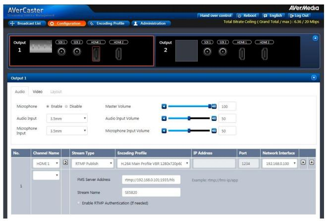
Then click on the "HDMI 2" icon to select HDMI port 2 for streaming. In this case we use TS Multicast to 224.2.2.2:1234.
