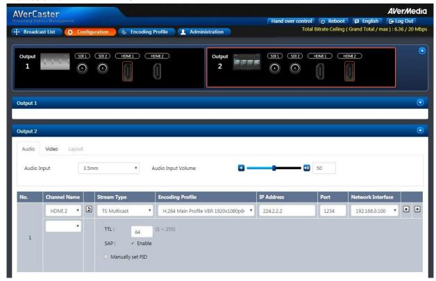
In the "Broadcast List" tab, you can see in "Channel Name" column that the two streaming tasks are coming from different video inputs. You can easily add one more video source to both Output 1 and Output 2 to achieve the scenario mentioned earlier.
