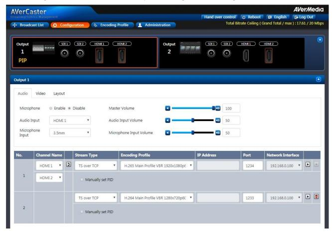
Below the highlighted Configuration tab are the input selection icons, which resemble the connectors in the back of SE5820. They give you an intuitive way of selecting video and audio inputs by clicking on the connectors.
