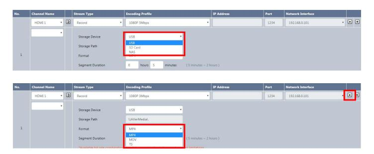
Note: Dropped frames may occur when using different types of external storages. We recommend using an HD/SSD speed test software, switching to another storage, or lowering your bit rate (e.g. 10 Mb) when it happens repeatedly.
