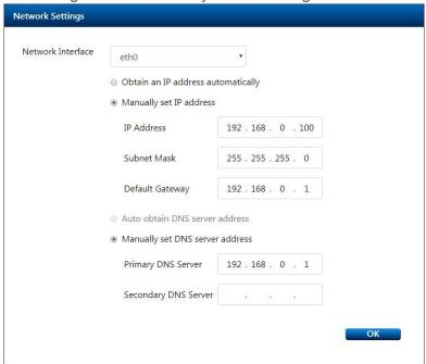
There are 2 network interfaces available for configuration on SE5820: LAN A and LAN B. If the cable is not connected, the IP address shows "0.0.0.0".
