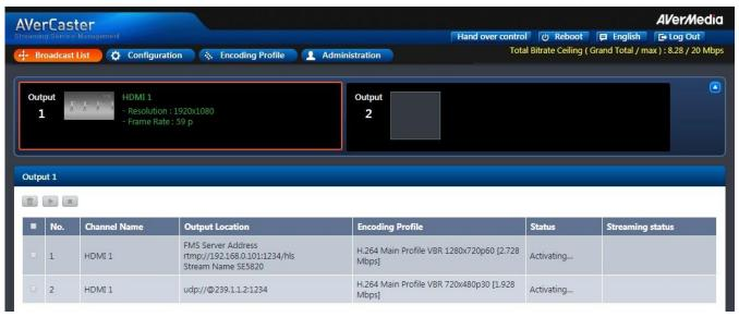
Note: Each Output supports up to 2 streaming tasks or 1 streaming and 1 recording task at the same time, however only 1 recording task can be perform at a time.
