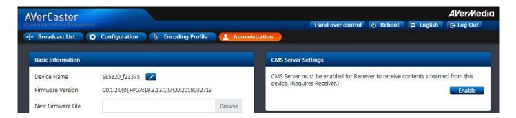
Click "Enable" in "CMS Server Settings". Enter the IP address and port number of the CMS server. CMS is installed to port 80 by default. Click "Connect" to link SE5820 to CMS server.
