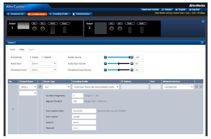
HLS delivers streaming with a playlist with file names ending ins "m3u8", such as "index.m3u8". The media itself is split into multiple segments of "\*.ts" files, which are described in the playlist. The number of segments and duration of each segments can be configured to meet your needs.
